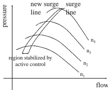
Fig. 5. Compressor map with effect of active control.
