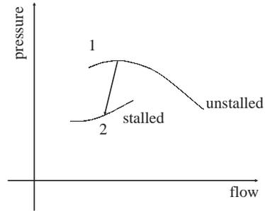
Fig. 1. Compressor map with stalled flow characteristic.
