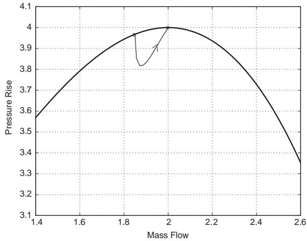
Fig. 13. Steady axisymmetric compressor characteristic: controlled transient response.
